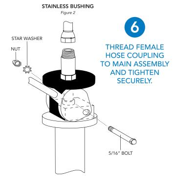
INSTALL 5/16" BOLT THROUGH ARM CAM AND BUSHING. INSTALL WASHER AND TIGHTEN NUT.
